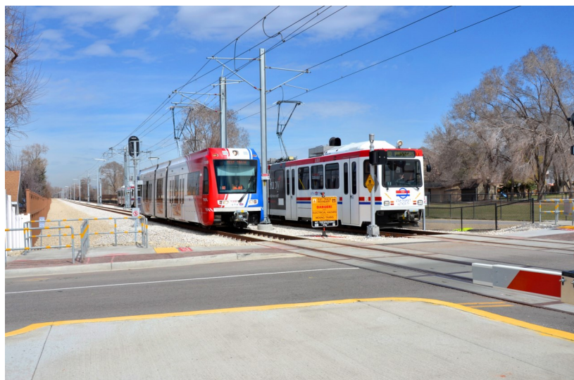
New S70 rail car (left) alongside the older SD160 rail car during systems integration testing on the Draper Line which is due to open in August of 2013
